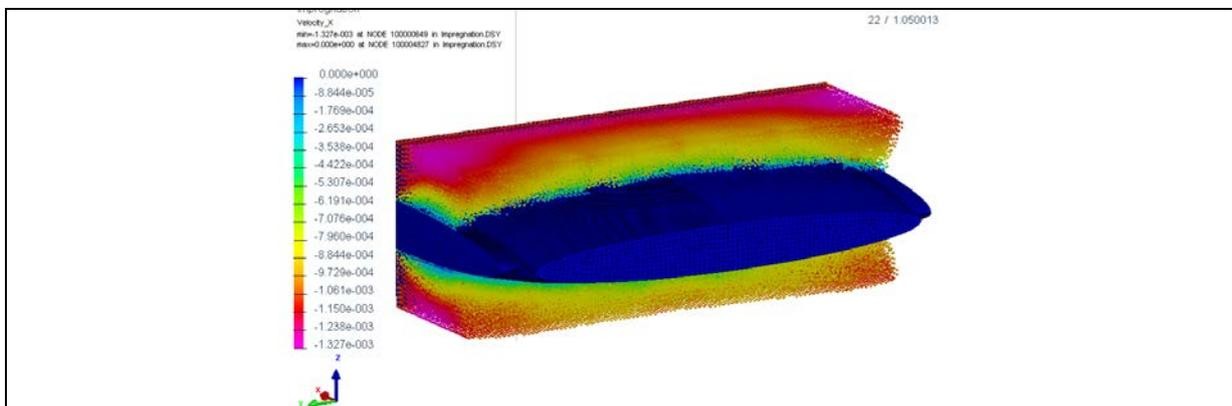
**Figure 3:** Impregnation of a plain weave unit cell at the meso level showing the velocity profile (m/s) during inflow with a constant velocity. A no-slip condition was used at the yarn interface surface and slip conditions at the other surface.
