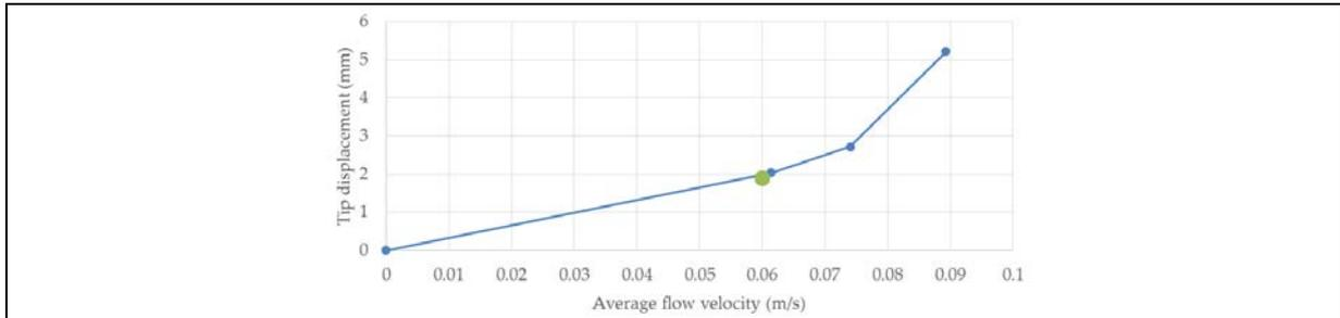
**Figure 2:** Experimental and modelling results. The graph shows the average flow velocity (m/s) versus the tip displacement of the rubber rod (mm). The blue line represents the experiments, the green dot the simulation results.
