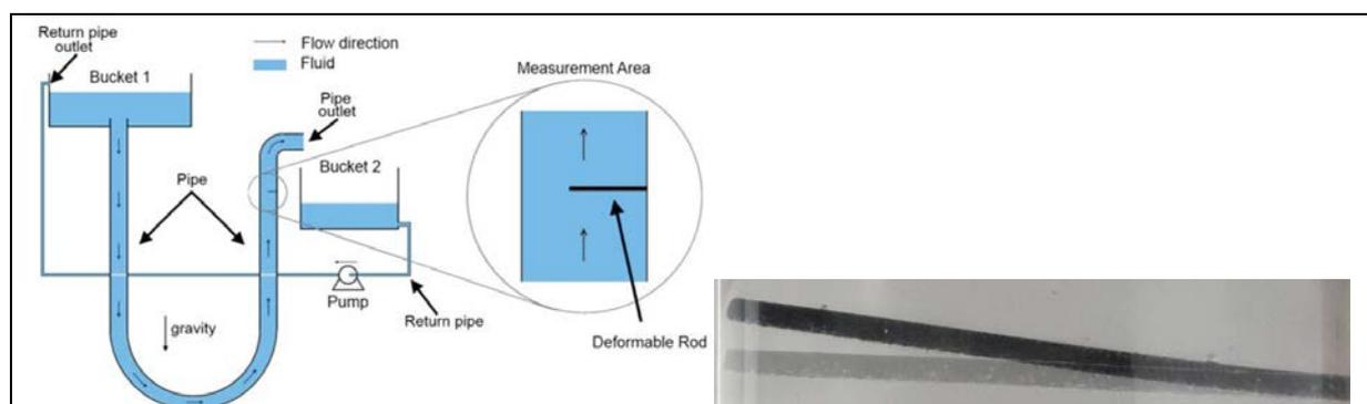
**Figure 1:** *Experimental set-up to measure the flow induced deformation of a rubber rod. The left hand side shows the schematic setup of the experiment while the right hand side shows the detail of the rod in the pipe during the experiment. The deformed (black) and undeformed (grey) shape are shown in the photograph.*
